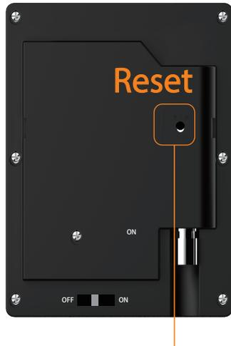
Keep the device on, prick the Reset hole for 5 seconds to restart the device.
